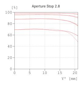
The MTF is indicated both at full aperture and at f/5.6 at long taking distances (infinity). Shown is the contrast in percentage for 5, 10, 20 and 40 lp/mm accross the height of the 35 mm film format, for tangential (dotted line) and sagittal (solid line) structures, in white light. The 5 and 10 lp/mm will give an indication regarding the contrast ratio for large object structures.The 20 and 40 lp/mm records the resolution of finer and finest object structures.
